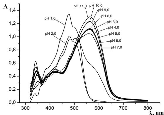
Fig. 3. Absorption spectra of toluene solutions of 1-(5-benzyl-2-thiazolyl)-azo-2-naphthol in the presence of  $\text{Co}^{2+}$  ions at  $\text{pH} = 1-12$ ;  $C(\text{Reag}) = 5.9 \cdot 10^{-5} \text{ M}$ ,  $C(\text{Co}^{2+}) = 3.3 \cdot 10^{-4} \text{ M}$ ,  $l = 1.0 \text{ cm}$
