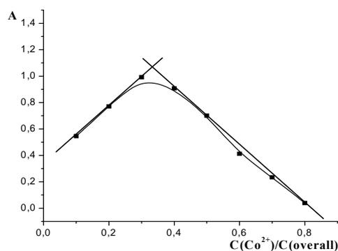
Fig. 5. Setting the ratio of the interaction in the system Co(II) – 1-(5-benzyl-2-thiazolyl)-azo-2-naphthol by the method of continuous variations;  $C(\text{total}) = 9.0 \cdot 10^{-5}$  M, pH = 12,  $l = 1.0$  cm,  $\lambda = 565$  nm
