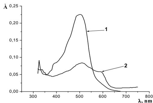
Fig. 6. The absorption spectrum of 1-(5-benzyl-2-thiazolyl)-azo-2-naphthol in toluene solution in the absence (1) and in the presence (2) of  $\text{Ni}^{2+}$  ions;  $C(\text{Reag}) = 1.5 \cdot 10^{-5}$  M,  $C(\text{Ni}^{2+}) = 7.5 \cdot 10^{-5}$  M,  $C(\text{NaOH}) = 8.0 \cdot 10^{-2}$  M,  $l = 1.0$  cm
