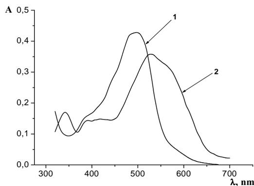
Fig. 2. Electronic absorption spectra of 1-(5-benzyl-2-thiazolyl)-azo-2-naphthol in the absence (1) and in the presence (2) of  $\text{Co}^{2+}$  ions;
