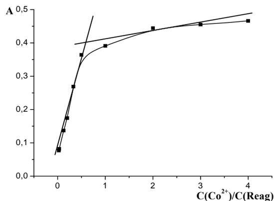
Fig. 4. Dependence of toluene extract optical density from the ratio of components in the system  $\text{Co}^{2+} - 1-(5\text{-benzyl-2-thiazolyl})\text{-azo-2-naphthol}$ ;  $C(\text{Reag}) = 5.8 \cdot 10^{-5} \text{ M}$ ,  $\text{pH} = 12$ ,  $l = 1,0 \text{ cm}$ ,  $\lambda = 565 \text{ nm}$
