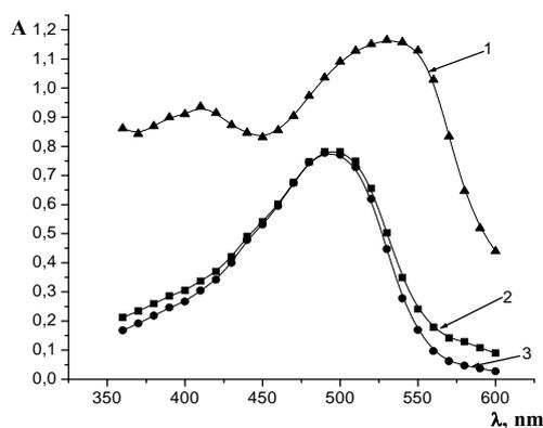
Fig. 7. The absorption spectrum of 1-(5-benzyl-2-thiazolyl)-azo-2-naphthol in toluene solution at the presence of  $\text{Ni}^{2+}$  ions in the initial solution after preliminary separation of nickel by triple extraction of its dymethylglyoksimate into chloroform,  $C(\text{Reag}) = 4,5 \cdot 10^{-5} \text{ M}$ ,  $m(\text{Ni}) = 2.2 \text{ mg}$  (1);  $0.44 \text{ mg}$  (2);  $0.22 \text{ mg}$  (3);  $C(\text{NaOH}) = 8.0 \cdot 10^{-2} \text{ M}$ ,  $l = 1.0 \text{ cm}$ .
